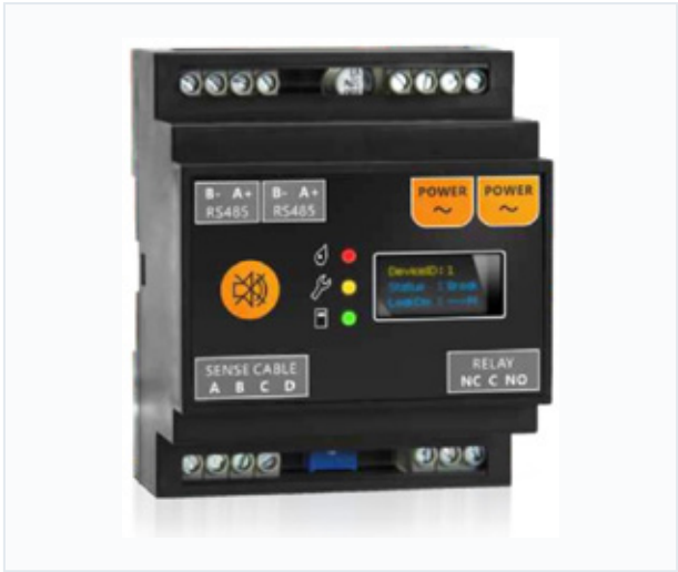
DIN-rail locating detection module. One sense-cable channel, position display, Modbus RTU over RS-485.
